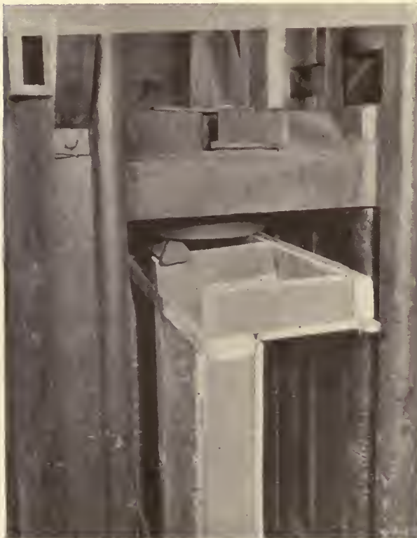
LOAD APPLIED ON CENTER STUD
